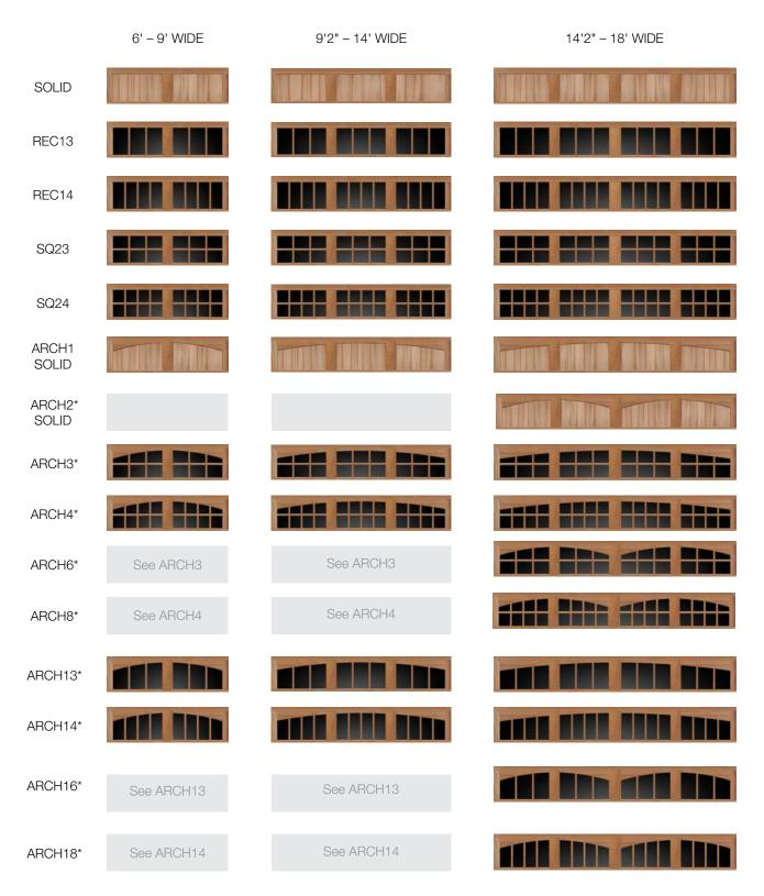
\* Arched windows available in 8', 9', 10', 15', 15'6", 16' and 18' widths ARCH3, ARCH4, ARCH6 and ARCH8 are not available in 7'6" high doors. 1/8" glass standard. Obscure glass is available as an option.
